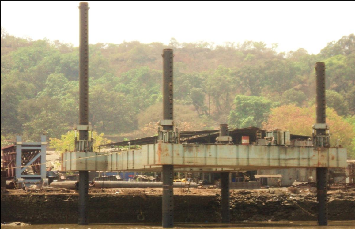
Modular Jack-up Barge made Under IRS Class. Size : 18 mtr x 18 mtr / 36 mtr Spud length
