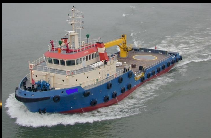
Offshore Supply Vessel – 10 mtr x42 mtr +12 4 crew built under RINA class
