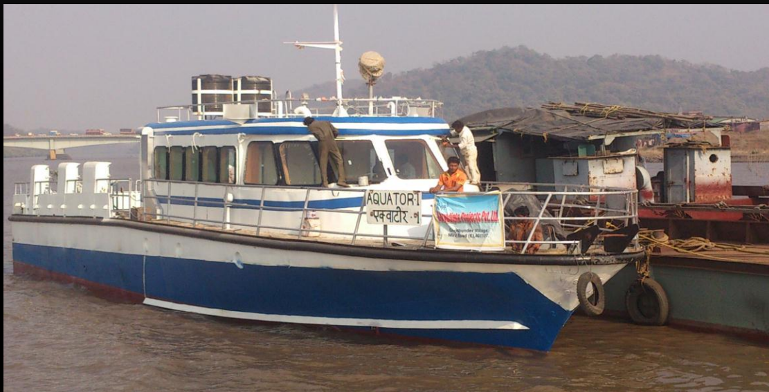
Aquator Crew Boat built by S.P.P.L under IRS class ,capacity 30 pax + 6 crew. Area of operation - 200 nautical miles from shore , complied under SPS code.
