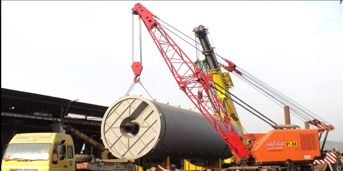
Desolventizer Toaster -: 4 mtr dia x 12 mtr 8 stage Exported to Russia
